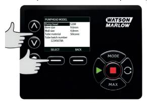
Use the A /V keys to move the selection bar over the required pumphead type and press **SELECT**.
