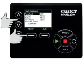
Use the  $\land \land \lor$  keys to move the selection bar over the tube material to be used and press **SELECT**.
