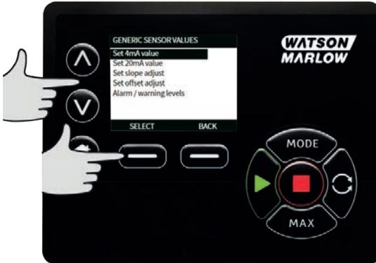
11. Using the  $\wedge/\vee$  keys, change the value reported when the sensor input is at 20 mA. Once satisfied with the value press **SELECT**.
