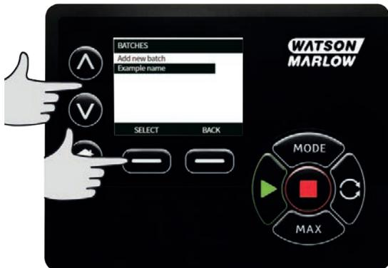
3. Press **SELECT** to edit a parameter. Set each parameter to the desired value. See "Batch parameters" on page 104 for a description of the parameters.
