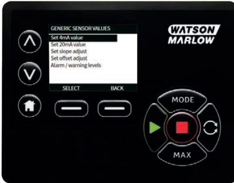
2. Using the  $\uparrow/\downarrow$  keys, scroll to **Set slope adjust**
