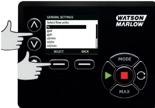
2. If a mass flow unit is selected, the specific gravity of the fluid must be entered. The following screen is displayed.
