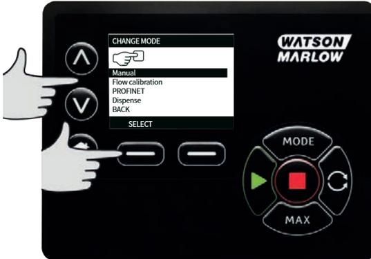
2. Using the  $\wedge$  /  $\vee$  keys, scroll to **DISPENSE** and press **SETTINGS**
