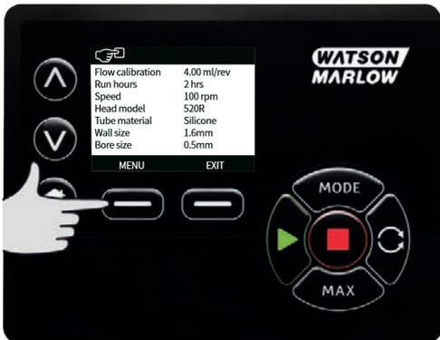
2. This will display the **MAIN MENU** as shown below. Use the  $\wedge$   $\vee$  keys to move the selection bar between the available options.
