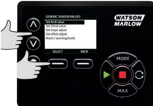
3. Using the  $\wedge/\vee$  keys, select the value to change and press **SELECT**.
