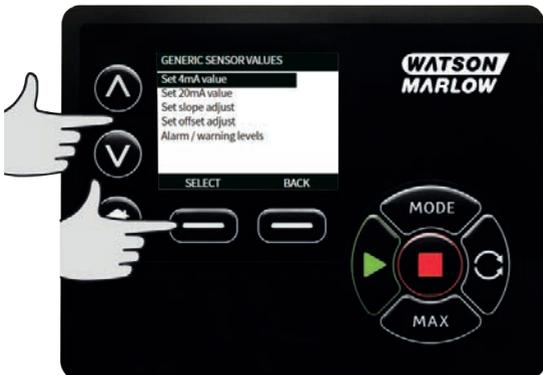
3. Using the  $\wedge/\vee$  keys, scroll to the desired value and press **SELECT**
