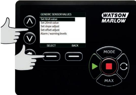
9. Using the  $\wedge/\vee$  keys, change the value reported when the sensor input is at 4 mA. Once satisfied with the value press **SELECT**.
