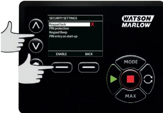
2. Once locked it will display the screen below when any key is pressed. To unlock the keypad press the two **UNLOCK** keys together.
