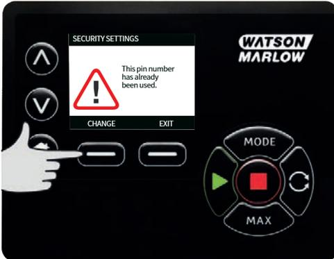
7. If the PIN entered does not allow access to the functionality the following screen will be displayed.
