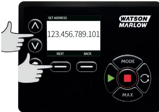
3. After setting the last number, press **CONFIRM** to store the number and return to the **ETHERNET/IP™ SETTINGS** screen.
