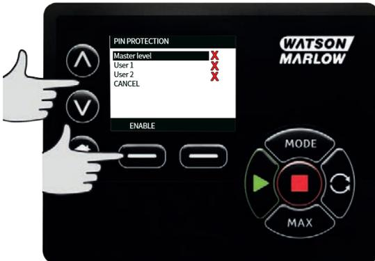
2. **ENABLE** user 1 security settings displays the PIN entry screen for User 1. To define a four digit User 1 PIN, use the **^** / **v** keys to select each digit from 0-9. Once you have the required digit press the **NEXT DIGIT** key. After selecting the fourth digit press **ENTER**.
