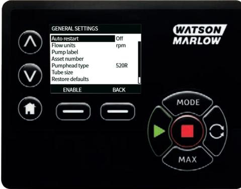
2. Using the  $\wedge$  /  $\vee$  keys, scroll to **Asset number** and press **SELECT**.
