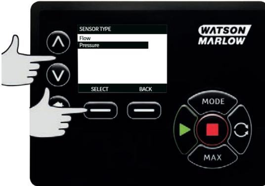
4. A list of supported flow sensor families are displayed. The example in the image above shows supported flow sensors. Using the  $\wedge$  /  $\vee$  keys, scroll to the desired flow sensor and press **SELECT**.
