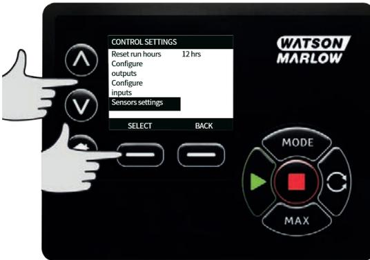
3. Using the  $\wedge/\vee$  keys, scroll to **Flow** or **Pressure** option and press **SELECT**. This selects the type of sensor to configure.
