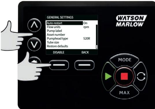
3. Use the  $\wedge$  /  $\vee$  keys to move the selection bar over **Pumphead** and press **SELECT**.
