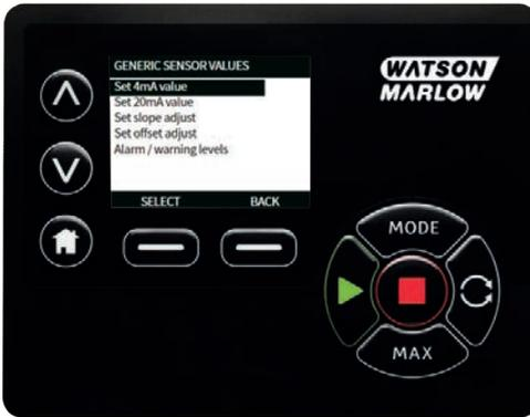
8. Using the  $\wedge/\vee$  keys, scroll to **Set 4mA value**
