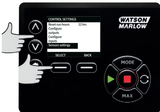
2. From the control settings menu, using the  $\wedge$  /  $\vee$  keys, scroll to **Set sensor delay** option and press **SELECT**
