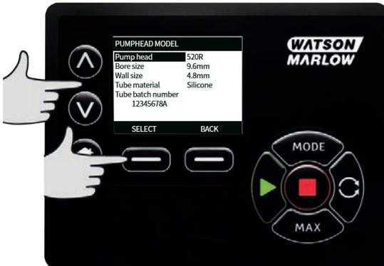
2. Use the  $\wedge$  /  $\vee$  keys to move the selection bar over the tube size to be used and press **SELECT**.
