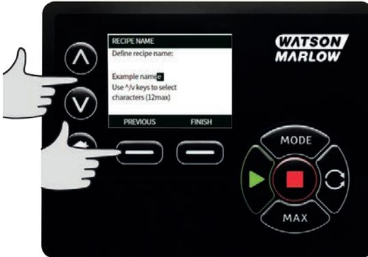
6. Use the  $\wedge/\vee$  key to highlight any of the remaining parameters and press **SELECT**.
