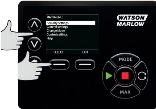
2. Use the  $\wedge$  /  $\vee$  keys to move the selection bar over **Pumphead type** and press **SELECT**. The following screen will be displayed.
