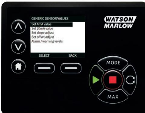
2. Using the  $\wedge/\vee$  keys, scroll to **Set offset adjust**
