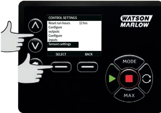
2. Using the  $\wedge$  /  $\vee$  keys, scroll to **Configure sensors** option and press **SELECT**.
