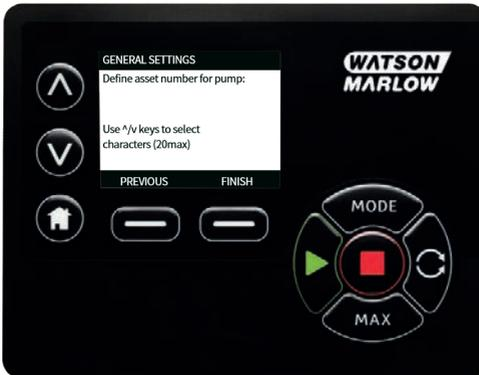
6. Power the pump off and on again to apply the asset number.
