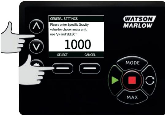
3. Use the  $\wedge$  /  $\vee$  keys to enter the value of the specific gravity, and press **SELECT**.
