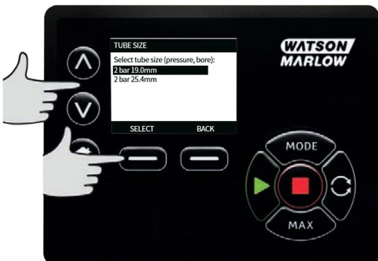
4. This screen also allows you to select the tube material used. Use the  $\wedge$  /  $\vee$  keys to move the selection bar over **Tube material** and press **SELECT**.
