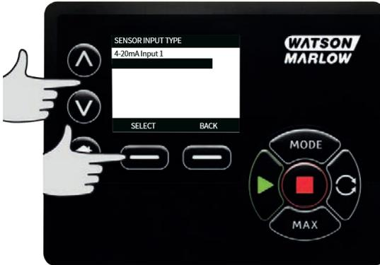
6. Using the  $\wedge$  /  $\vee$  keys, scroll to the desired flow sensor and press **SELECT**.
