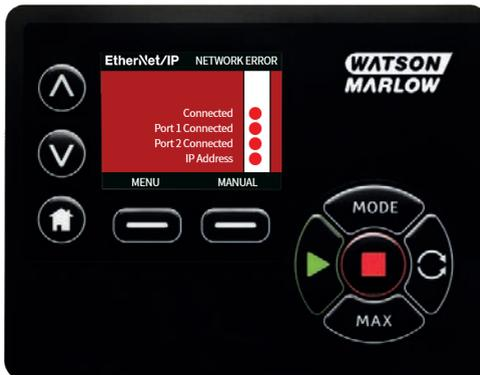
3. If the pump is connected to a PC, press **INFO** to display the network settings.
