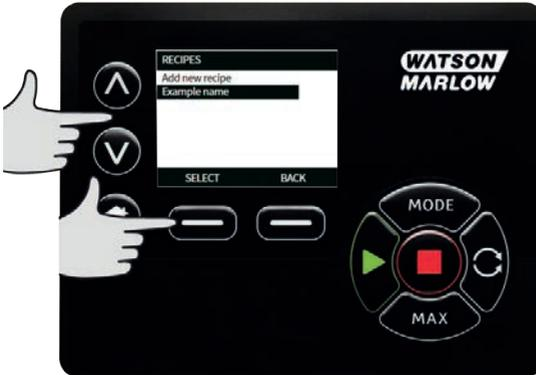
Press **SELECT** to edit a parameter. Set each parameter to the desired value. See "Recipe parameters" on page 105 for a description of the parameters.
