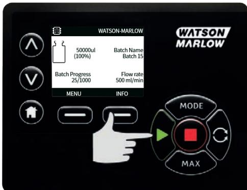
Starts the pump, and the display background changes to grey. If the pump is already running, pressing this has no effect.
