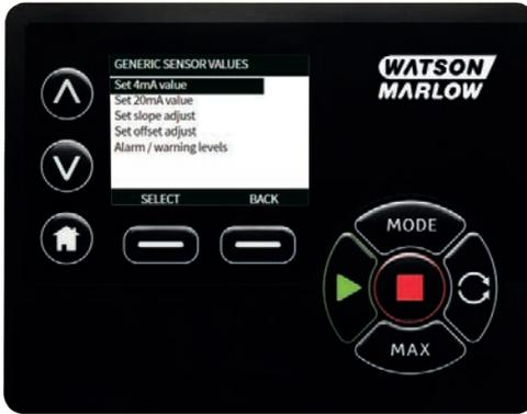
2. Using the  $\wedge/\vee$  keys, scroll to **Alarm / warning levels**
