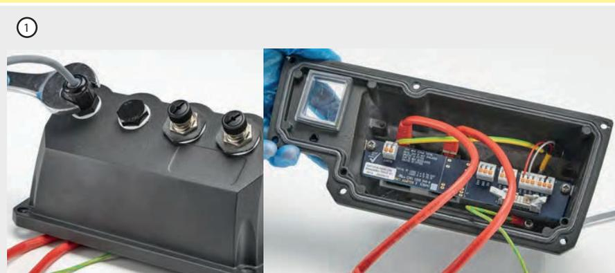
Control cable earth screening connected to Earth terminal (J6) on adapter PCB when plastic cable gland is used.
