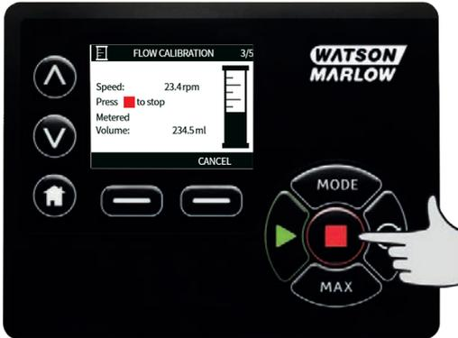
5. Use the  $\wedge$  /  $\vee$  keys to enter the actual volume of fluid pumped.
